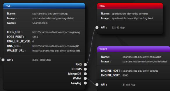
Backend Wallet Architecture is used when the RGS Server is placed in front of a Wallet, receiving Bet requests from Game Clients directly. In Backend
